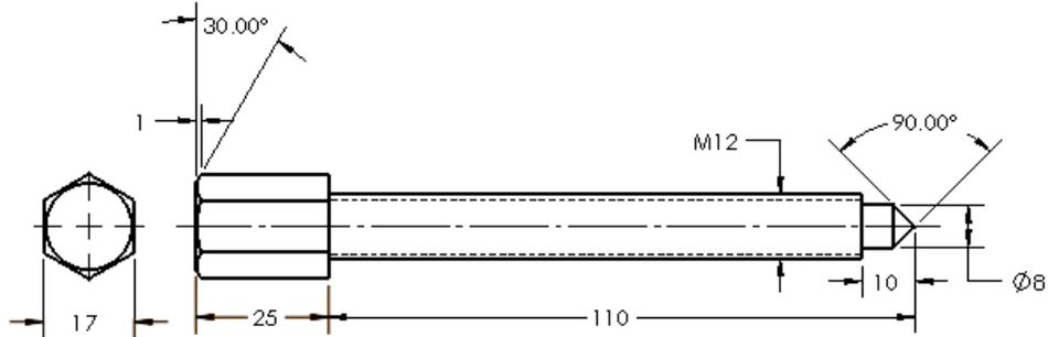
We will create the rod with the thread and the pointed end as a rotation form. The hexagonal part will be added to this as an extrusion.
