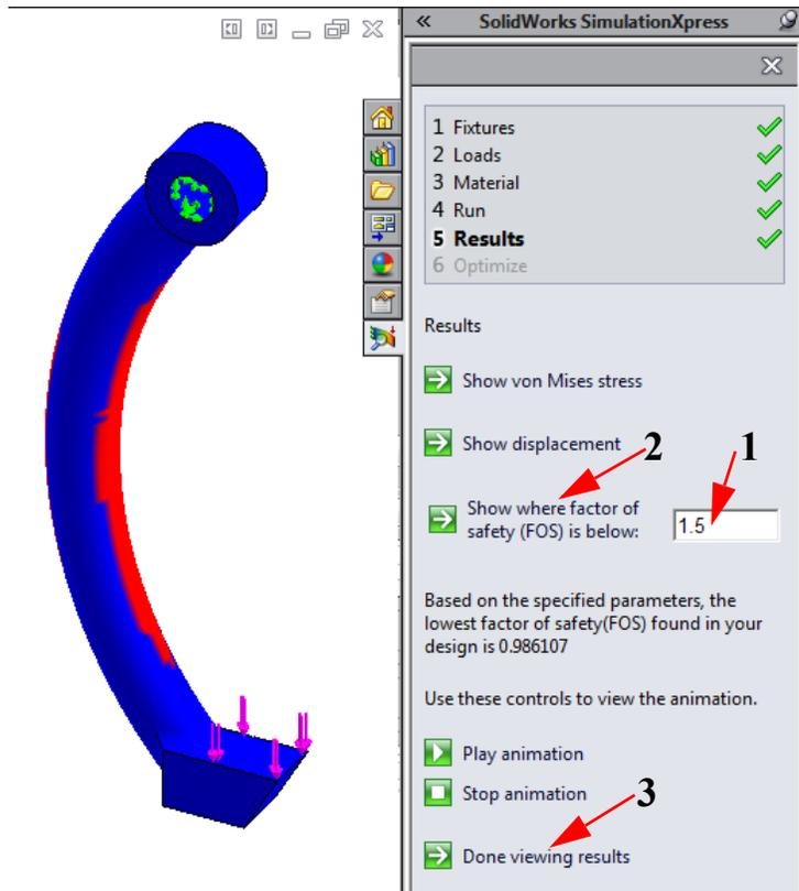
93 We can strengthen the part by decreasing the curve of the arm, so the radius will increase. We improve the model to get a FOS value of 1.
