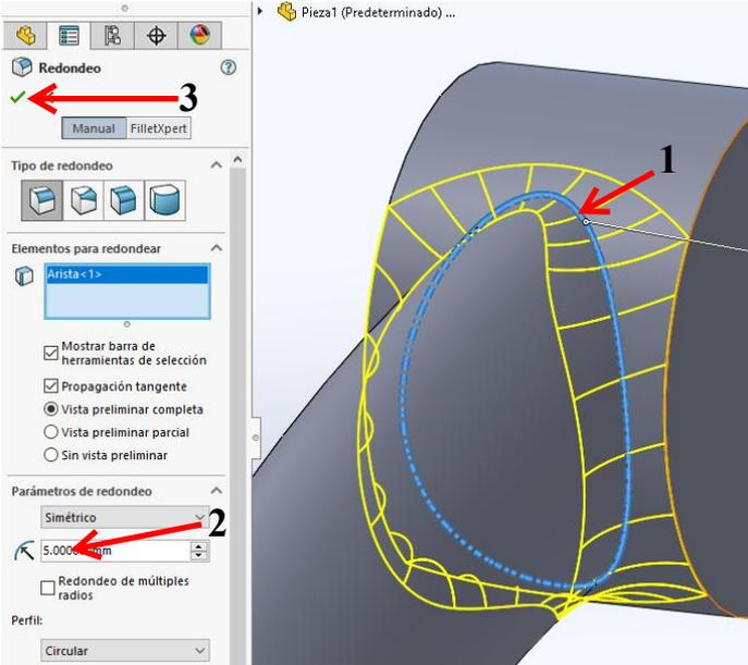
84 Next, round off the connection at the bottom. Click on **Fillet** in the **CommandManager**. Select both cutting lines now. The radius is also set to **5 mm**.
