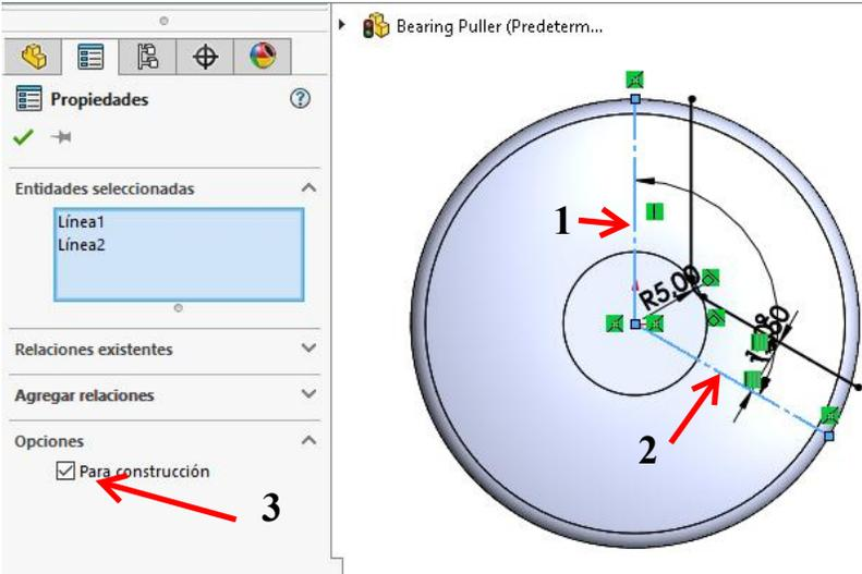
**Tip:** We have also used centerlines in other tutorials. These lines are actually auxiliary lines. When you use a sketch to make an extrusion, for example, SolidWorks only uses the 'real' lines and not the auxiliary lines.
