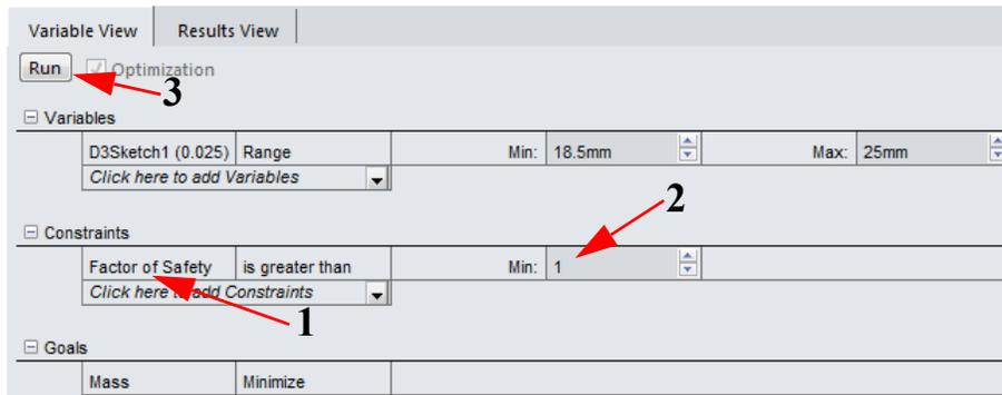
62 SimulationXpress has calculated that the model height can be reduced to 18.5 mm and still have a FOS of 5.49. The weight has been reduced by 30%, from 381 grams to 265 grams.
