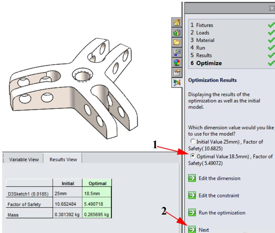
**Note:** The factor of safety is still above 1. However, the height of the part cannot be reduced without changing the hole locations. Other dimensions can be changed in order to reduce the factor of safety even more.
