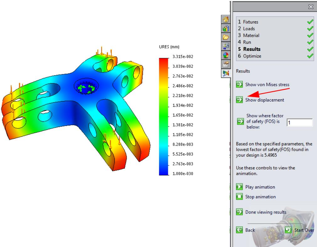
66 You can now see how the model distorts (exaggerated display) under the influence of the force.
