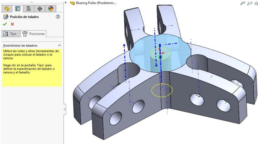
**Tip:** When you have to place a hole using the Hole Wizard (steps 37-38), you are actually making a sketch. By putting a point in that sketch, you are positioning the hole.
