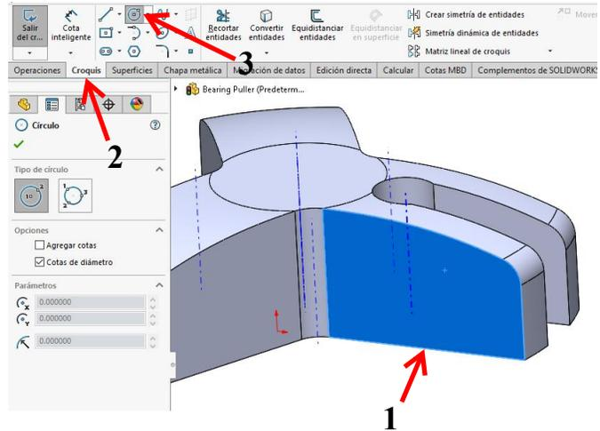
28 Rotate the model with **Normal To**, and draw two circle at random positions like in the drawing on the right.
