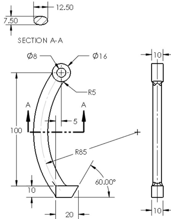
We will build this model by shaping the upper circle and lower part of the finger and will add the arm as a **sweep** later.
