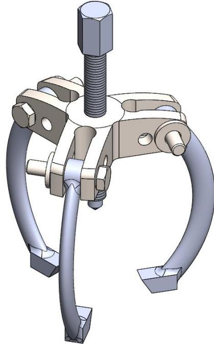
119 Finally, we need to place the nuts. Use **DIN > Nuts > Hex Nuts** from the **Toolbox**.
