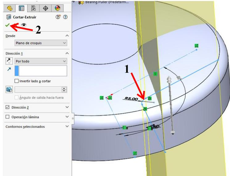
**Tip:** In most cases you will use a closed sketch for an **Extruded Cut**. In the case of a circle or a square, you will only make a hole in the shape of that sketch.
