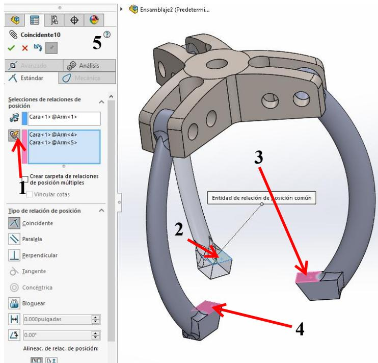
116 Finally, we have to put the bolt in position. Create a mate between the surfaces as illustrated on the right.
