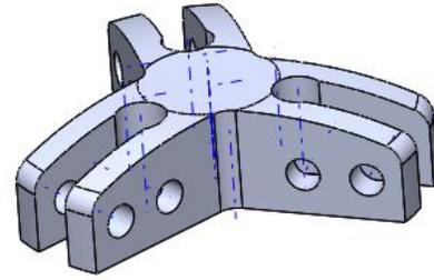
37 Set the hole on the top plane of the bridge at a random position.
