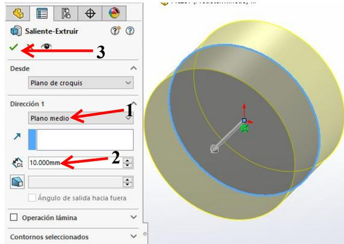
**Tip:** We have not use the **Mid Plane** option before. This tool is very convenient when you want to build a symmetrical model. The sketch will extruded equally wide in two directions.
