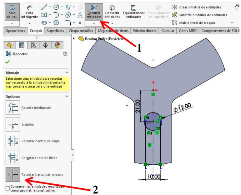
24 Next, click on the parts of the sketch that must be removed. Make sure you end up with a sketch similar to the one on the right.
