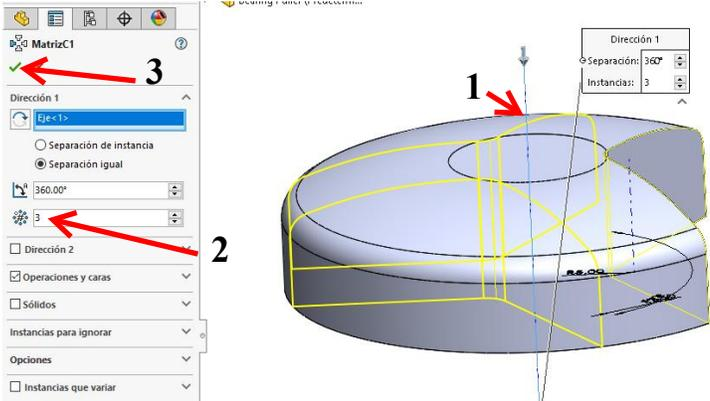
**Tip:** Notice that in the three last steps we first selected the feature in the **FeatureManager** and then selected the **Circular Pattern** command. At this point, SolidWorks ‘understands’ that you want to use this command for the selected item and automatically adjusts the settings in the **PropertyManager**.
